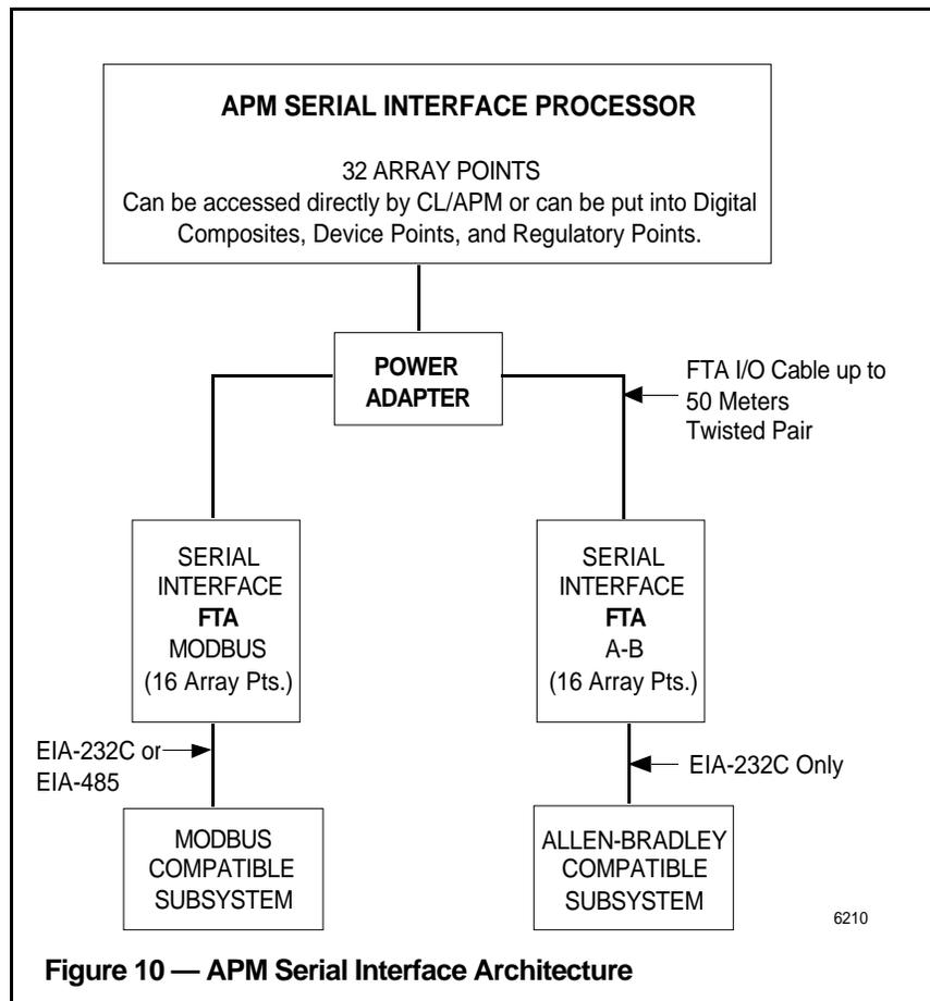
**Figure 10 — APM Serial Interface Architecture**
