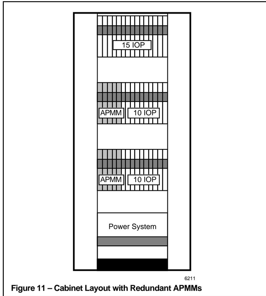
Figure 11 – Cabinet Layout with Redundant APMMs
