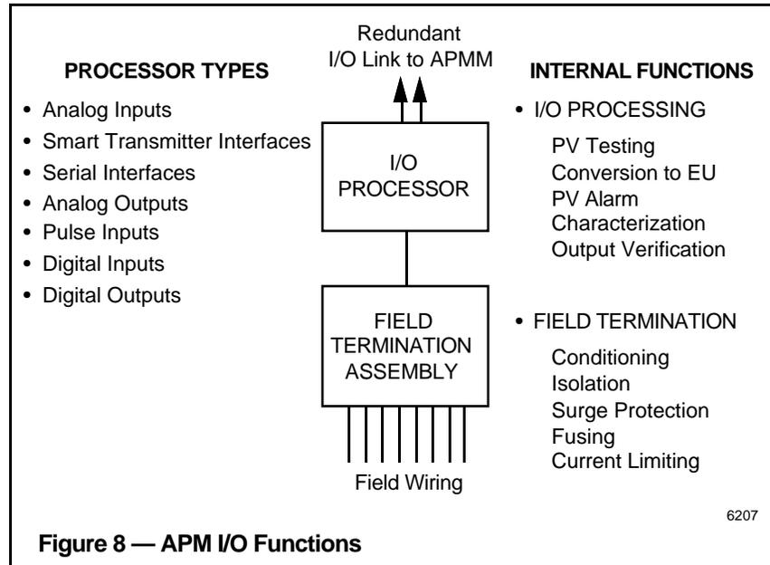
While a separate Field Termination Assembly of a given type is required to handle varying field wiring signal levels, identical I/O Processors can be used. This I/O approach simplifies system hardware selection and minimizes spare parts requirements. For example, there is one Digital Input Processor that can handle 24 Vdc, 120 Vac, or 240 Vac, depending on the FTA selected.
