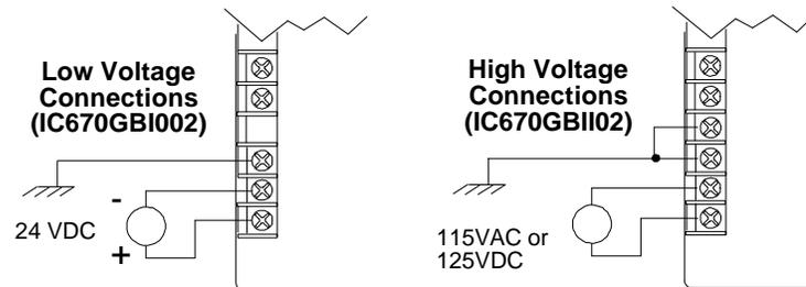
For BIU version IC670GBI102, if a DC supply is used the polarity is not important.
