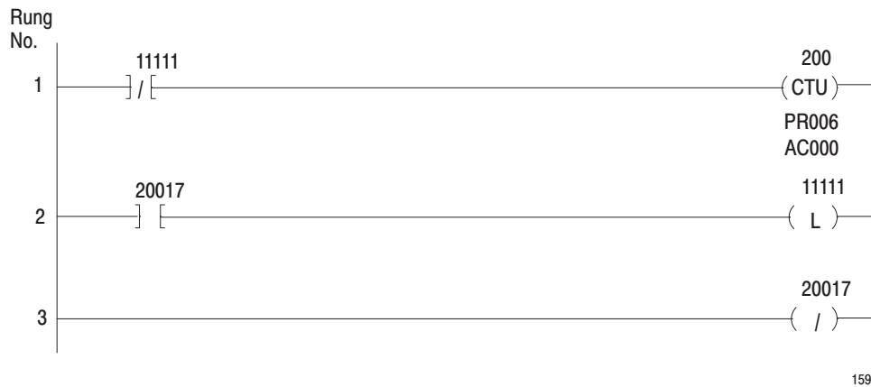
Figure 5.7 Scan Counter - PLC Processor
