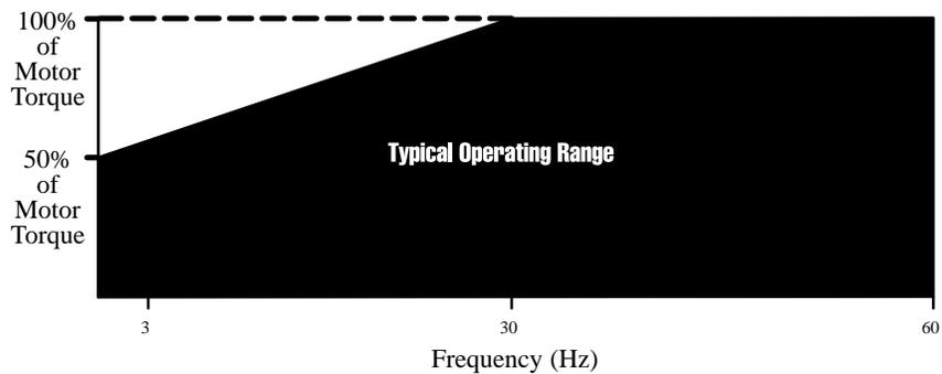
Shown above is a typical curve plotting torque versus speed. At slow speeds, if torque requirements continuously exceed levels shown above (10 minutes or longer), a motor rated for the required speed and torque range must be used. To guard against mechanical problems, it is recommended that the entire drive train machinery be checked for various limitations due to the range of the Bulletin 1336.
