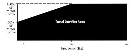
Shown above is a typical curve plotting torque versus speed. At slow speeds, if torque requirements continuously exceed levels shown above (10 minutes or longer), a motor rated for the required speed and torque range must be used. To guard against mechanical problems, it is recommended that the entire drive train machinery be checked for various limitations due to the range of the Bulletin 1336.
